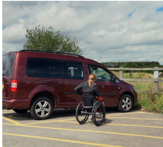
An accessible car parking space on firm, level surfaced ground with access zones marked out to the side and rear.
