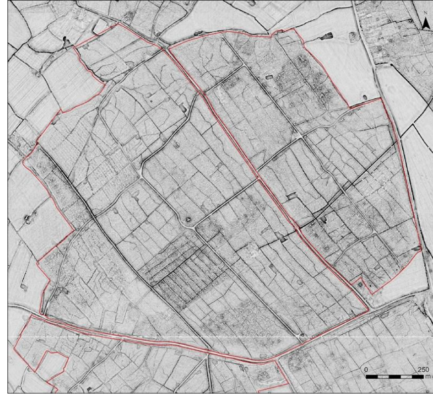
Figure 6 Openness Positive visualisation of lidar DTM for the northern half of Orlestone Forest, showing numerous small ponds and overlying patterns of drainage systems (darker features). Red line = boundary of Forestry England land. © Environment Agency 2018.
